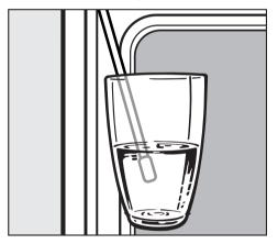
Hold a container with the quantity of water specified under the tube as shown. Start the water intake process with "OK". The amount of water required will be drawn up into the oven. As the water is taken in, bars will appear in the display. The amount of water specified will be more than the amount which is actually needed which means that some of the water will remain in the container at the end.
